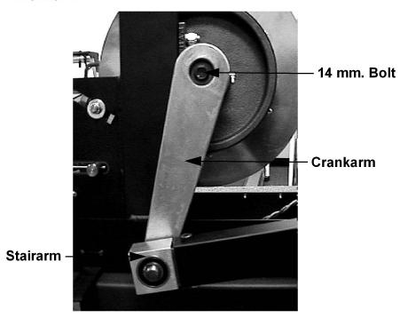
6. The crankarm removed from the right hand side has a magnet in a recess on the lower backside of the crankarm. The magnet is held in the crankarm by itis magnetism. Remove the magnet either by prying it out with a thin bladed screwdriver or by placing a heavy piece of steel near the magnet and allowing the it to adhere to the heavy piece of steel.
